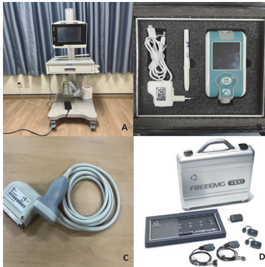
Fig. 1. Measuring equipment. A: Ultrasonography B: Myotone C: Ultrasonography Probe D: EMG
