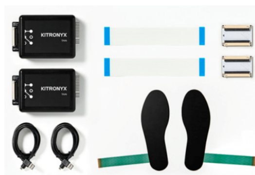
Fig. 2. KITRONYX components to provide real-time visual plantar pressure.
