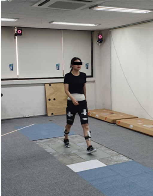
Fig. 1. Dynamic motion capture system with eight infrared cameras and two force platforms to obtain the 3D kinetic data during gait.
