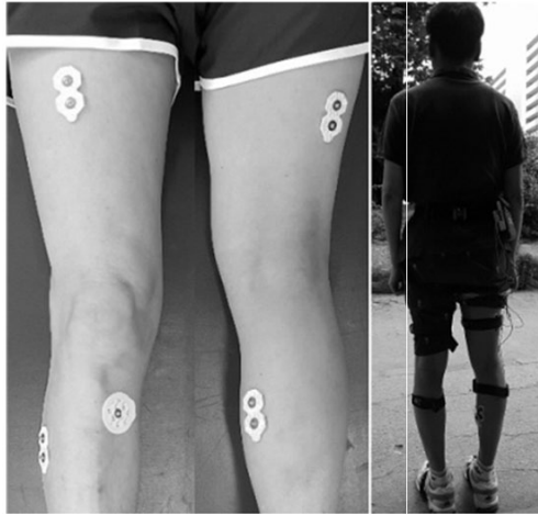
Fig. 3. Attachment of electrodes
