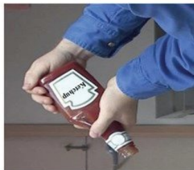
Ketchup is a good example of a thixotropic substance. It does not flow even when the bottle is held upside down.
