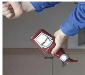
However, when the bottle is struck (vibrated), the ketchup temporarily liquefies and flows.
