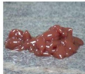
Once the vibration stops, the ketchup returns to its original viscous state.
